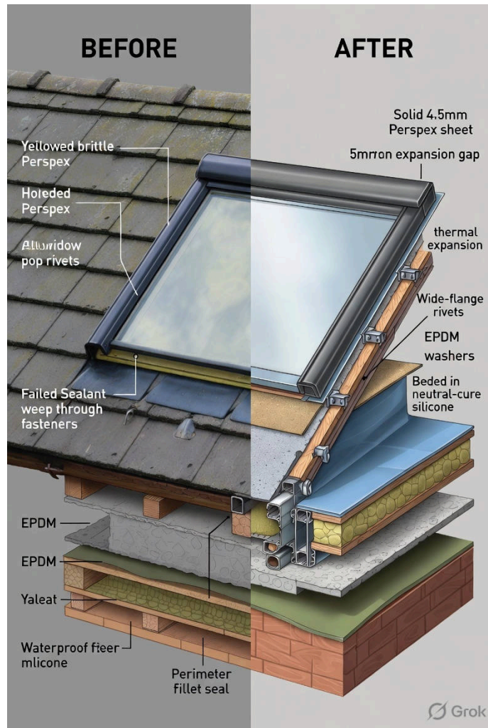
Diagram 1: Explaining the Job – Skylight Perspex Retrofitting Cross-Section
